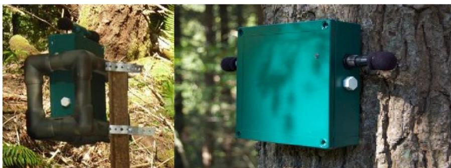
FIGURE 1.2: Left: A Song Meter recording device in H.J. Andrews. Right: An alternative microphone configuration.
